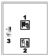
Correct hydrant's marking
