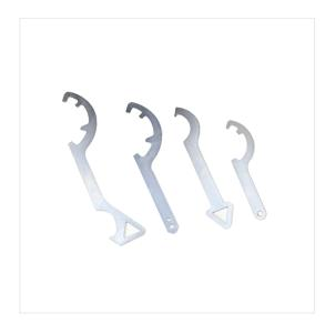
The wrenches are produced on a laser cutter, made of steel in the St3S grade, and powder paint.
