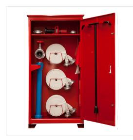
Universal cabinet for fire-fighting equipment It allows storing: pressure hoses, hydrant stand, key for gate valves, fire blanket. In addition, it allows the storage of small fire protection equipment type: nozzles, keys for connectors, switches, etc. **DIMENSIONS:** Height: 1440 - 1470 mm Width: 700 mm Depth: 350 mm
