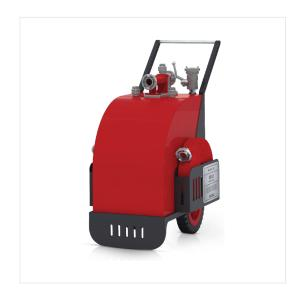
They are used in areas with risk of hydrocarbon fire such as car parks, refineries, aircraft hangars, airports, paint varnish workshops, filling stations, etc. They provide high extinguishing and cooling capabilities in fires caused by fuel, paint, etc. thanks to its film-forming foam concentrate. **DIMENSIONS:** Height: 1180 mm Width: 660 mm Depth: 1020 mm
